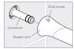
Tighten the grub screw using the hex key.
