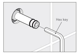
Carefully slide the shower arm over the connector and against the wall, make sure that the outlet on the end of the shower arm is pointing downwards and the grub screw is on top.
