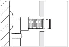
The distance between the wall and the end of the connector should be 13.5mm.
