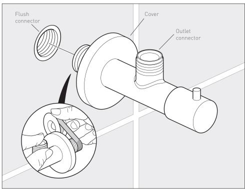
Using PTFE tape on the thread screw the valve into the connector. Make sure that the outlet is appointing upwards.
