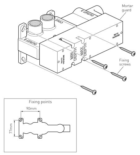
Select the position for the shower valve and offer the shower valve to the wall, make sure the valve is vertical with a level and mark the 4 fixing points with a suitable pencil, see above left for dimensions. Remove the shower valve from the wall, drill the holes to a suitable depth for the wall plugs and secure with suitable screws.
