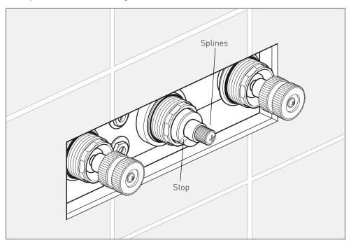
The valve has been factory set under balance pressures and hot water supply at 65° C. When your specific operating conditions are significantly different from the above, the temperature of the water may vary from the setting.
