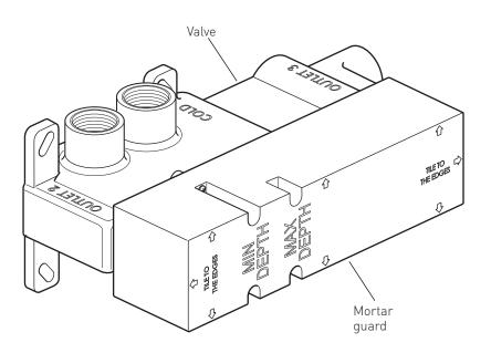
Rinse pipe work thoroughly before fitting the valve.
