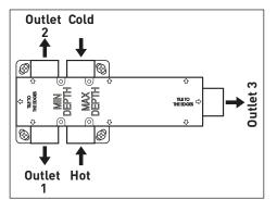
Finish the wall by tiling up to the mortar guard, keep the final finished wall surface between the min and max marks.
