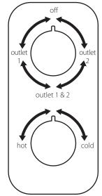
Turning the bottom handle anti-clockwise will increase the water temperature.
