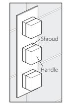
Please note: if the handle/shroud assemblies do not align, remove the offset spline and replace the other way up.
