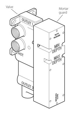
Rinse pipe work thoroughly before fitting the valve: do not allow dirt, metal particles or shavings to block the filters fitted on inlets.
