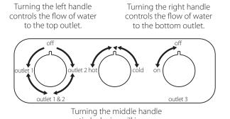
anti-clockwise will increase the water temperature. Installation - preparation
