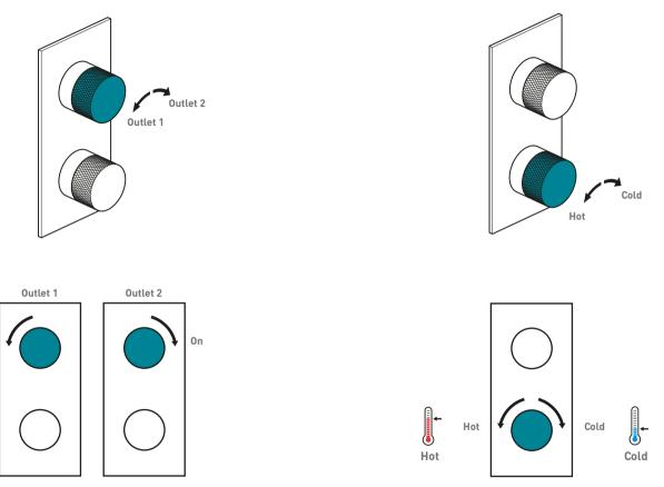
Turning the flow control handle in the direction of the arrow increases the flow of water to the outlet.
