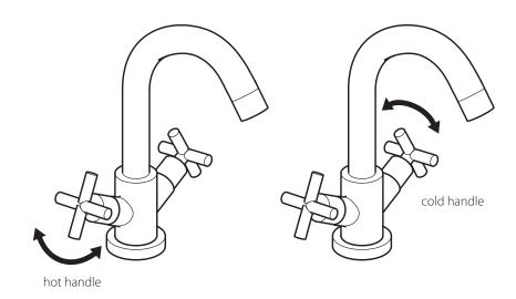
Turn the handles clockwise to increase the flow of water and anti-clockwise to decrease the flow.
