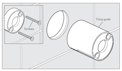
Remove the 2 screws using the suitable hex key provided with the ZON-128 and pullout the tiling guide.
