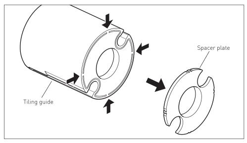
There is a spacer plate incorporated into the end of the tiling guide. Remove this by snapping it at the four points. Remove any burrs.
