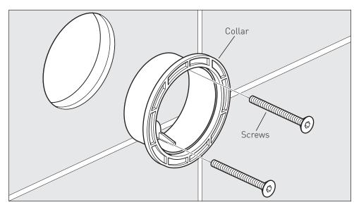
Slide the collar into the hole. Line up the holes and secure in position using the screws from the previous step.
