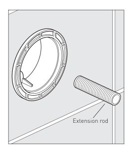
Screw the extension rod onto the spindle of the cartridge.
