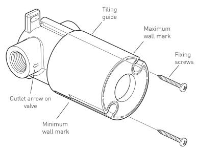
Select the position for the shower valve and offer the shower valve to the wall, make sure the valve is level and mark the 2 fixing points with a suitable pencil. Remove the shower valve from the wall, drill the holes to a suitable depth for the wall plugs and secure with suitable screws.
