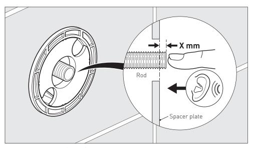
Measure the distance **(X mm)** the rod protrudes from the level of the spacer plate and then unscrew the rod and remove the spacer plate. **Note:** Ensure the cartridge is pushed in (the off position).
