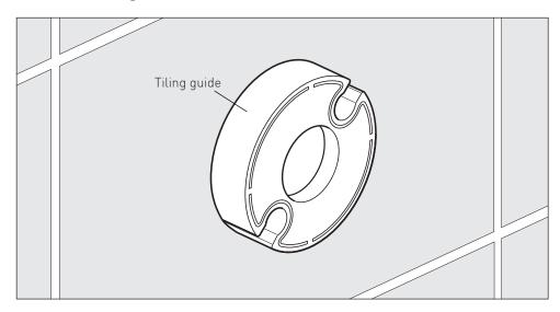
Tile around the tiling guide as tight as possible. Keep the final finished wall surface between the min and max marks.
