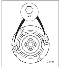
Make sure the cover is level and tighten the screws using the suitable hex key provided with the ZON-128 to secure the cover.
