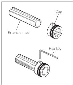
Screw the cap onto the rod until it's flush and tighten the grub screw on the cap using the smaller hex key provided with the ZON-128.
