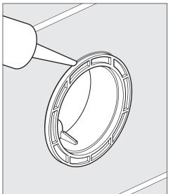
Apply a thin bead of silicone between the collar and the tiles.
