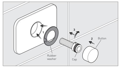
Fit the rubber washer, place the button onto the cap of the extension rod and screw the rod onto the spindle of the cartridge.
