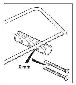
Cut away the measured distance **(X mm)** from the end of the rod as well as the 2 screws provided with the ZON-143 trim.
