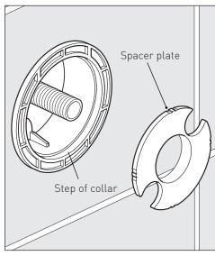
Insert the spacer plate into the step of the collar.
