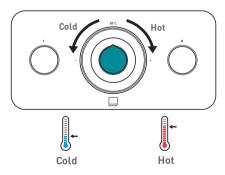
Turning the temperature control handle in the direction of the arrows increases/decreases the temperature
