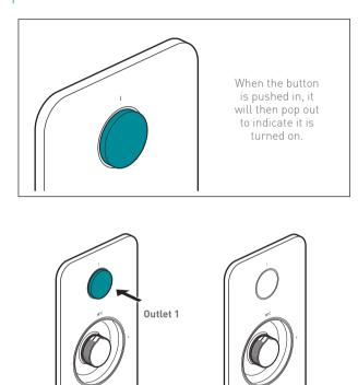
Pressing the flow control button turns on the flow of water to that outlet.
