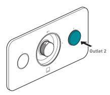
Pressing the flow control button turns on the flow of water to that outlet.
